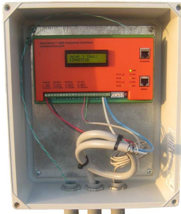
An Installed EtherMeter™ AMR-Industrial Interface
