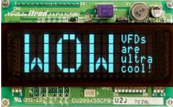
The VFD-420 Vacuum Fluorescent Display, Manufactured By SEETRON.
