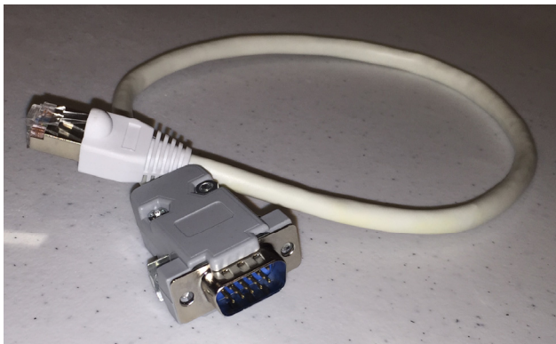
Figure 1. Custom Cable For Connecting the B202 Modem to the TM-2000/8000 Radio.
