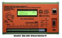
This can be accomplished using SCADAmetrics' model MTP "Milliamp-to-Pulse Converter", which converts an input 4-20mA signal into a pulse-output signal. This pulse output is then fed into an EM.100 EtherMeter, which counts the pulses and makes both total and rate information available to a connected SCADA system, AMI system, or both<sup>(1)</sup>.
