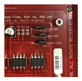
When using this Radio-Read Filter in **Non-EtherMeter Applications**, the Jumper Settings should be set to the following:
