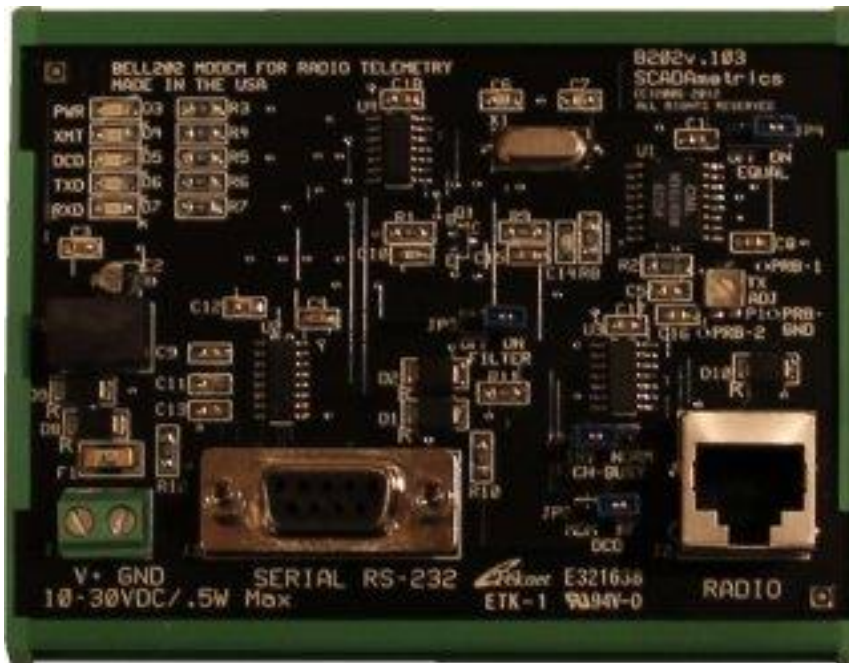
SCADAmetrics Bell-202 Modem For Radio Telemetry Model No. B202
